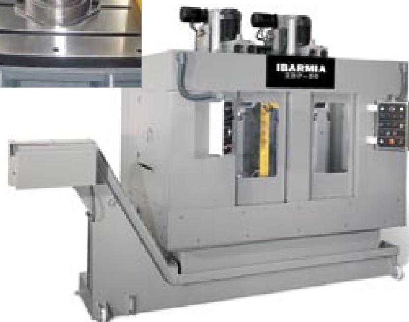
2 Headstock drill battery including full guarding, automatic doors, working area division, synchronized clamping tools, automatic chip conveyor and outside control panel.
