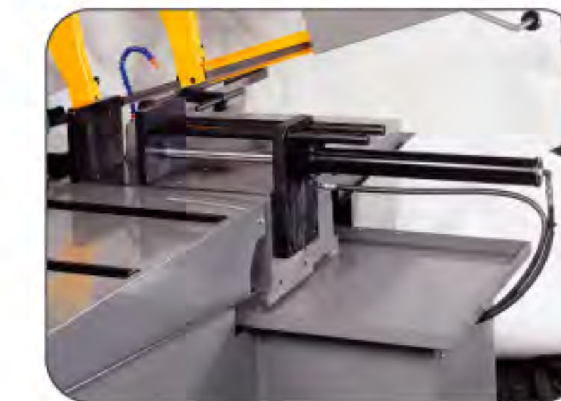
Hydraulic vise with two auxiliary rods for stable clamping
