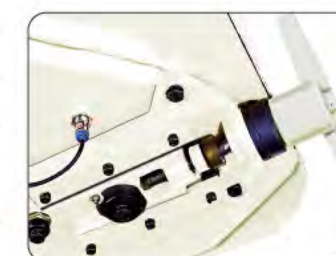
Manual blade tension device with automatic shut off device for saw blade breakage.
