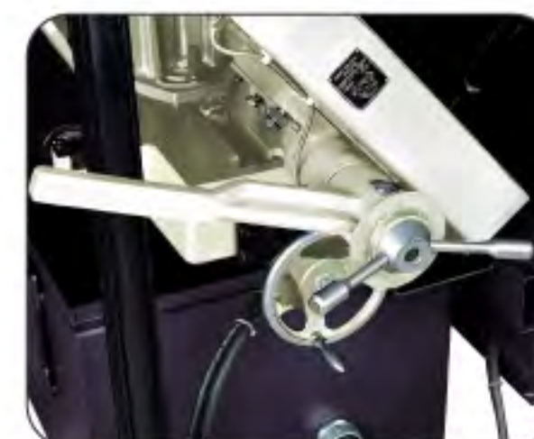
A large handle for quick setting the proper blade tension
