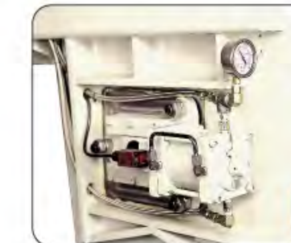
The device has function of saw blade breakage protection.
