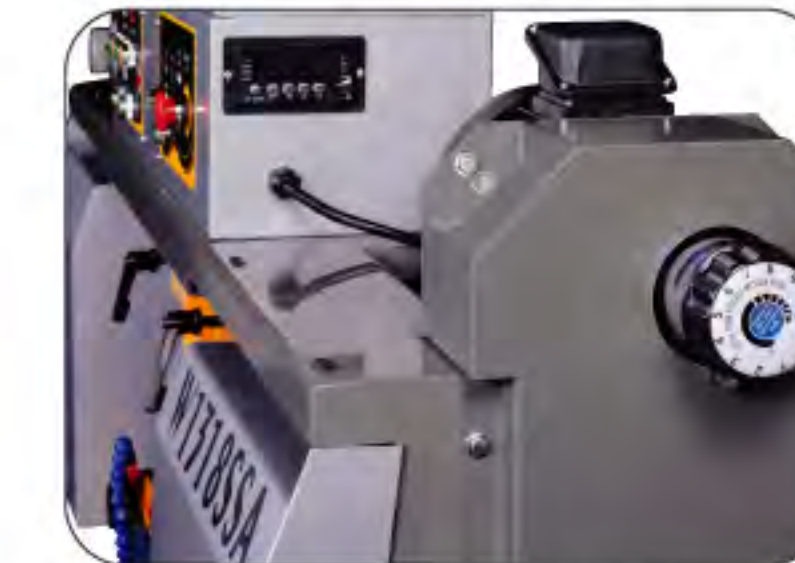
Variable speeds and digital blade speed display(BMT1318SSAV)
