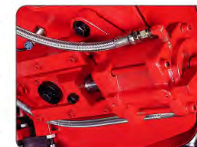
Hydraulic blade tension device with automatic shut off device for saw blade breakage
