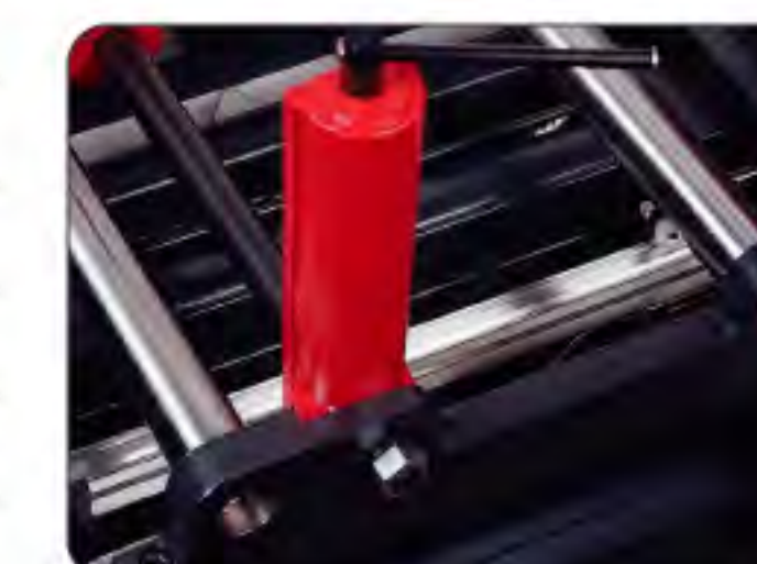
Linear scale for feeding material (BMT 330FANC)
