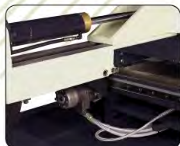
Hydraulic clamping vise and automatic position shifting.
