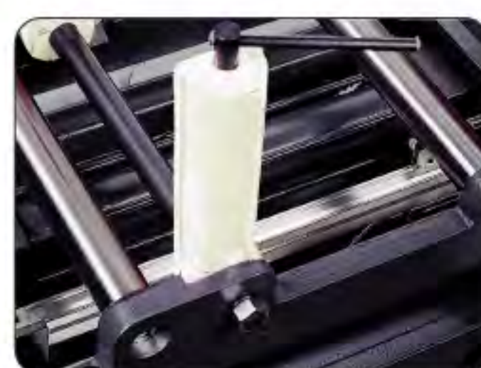
Linear scale for feeding material. (BMT 250FANC)
