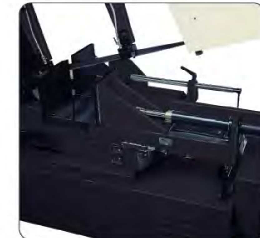
Hydraulic clamping vise-rigid, durable and stable
