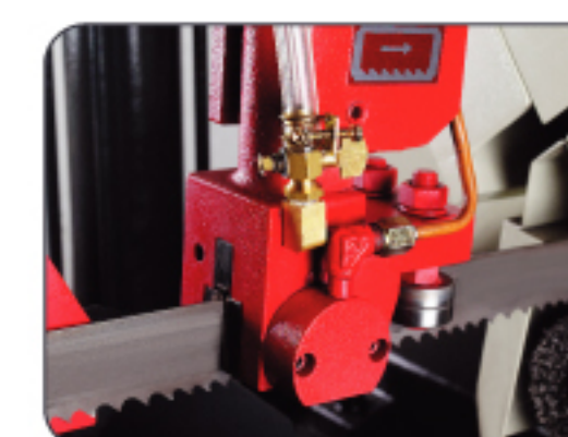
Hydraulic guiding device of saw blade
