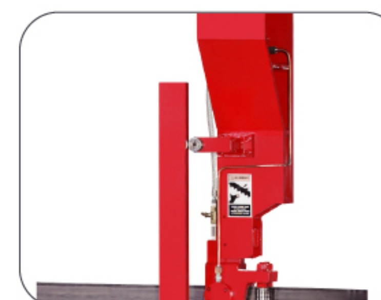
Synchronized adjustment of blade guide
