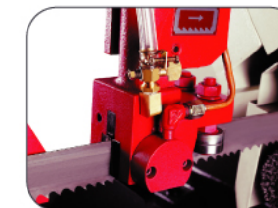
Hydraulic guide device of saw blade
